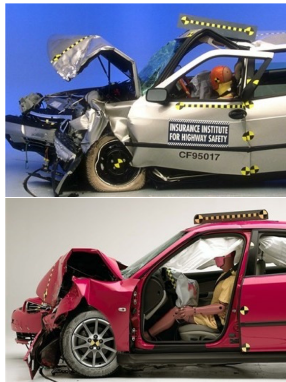
Figure 2. Occupant compartment collapse in the 64 km/h offset crash test, 1995 Saab 900 (top). Redesigned Saab 9-3, with occupant compartment essentially undamaged (bottom).
