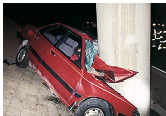
Figure 4. High speed crash into a concrete support pillar.
